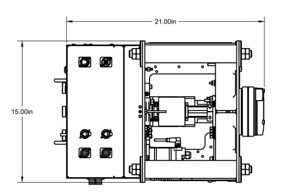
MOUNT HOIST WITH MINIMUM (2) -CHEESEBOROUGH CLAMPS, (1) ON EACH INDICATED TUBE MEMBER. ADJUSTED SO THAT LINE DROPS STRIAGHT OFF DRUM.
